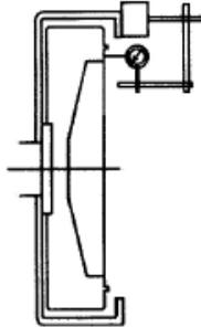
**4.6 Check engine crankshaft endplay.**
